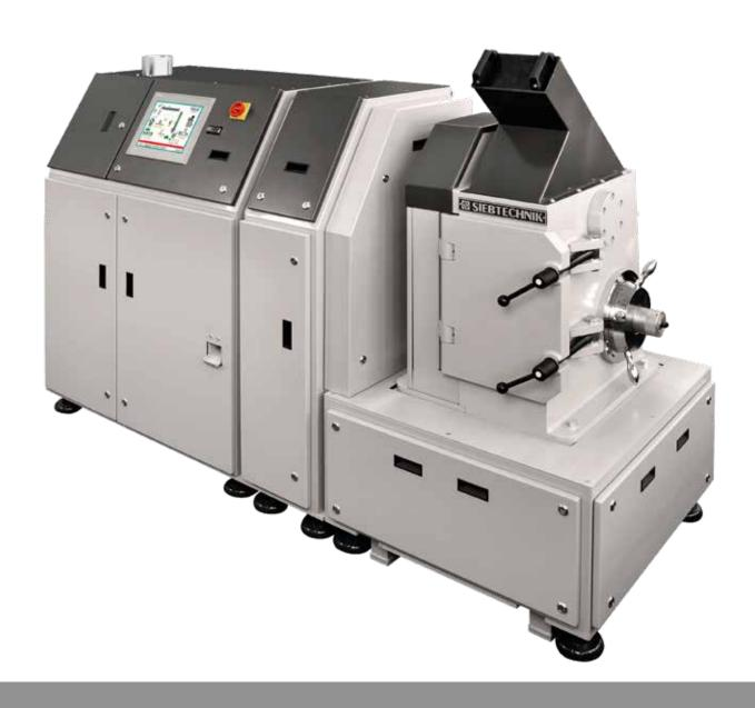
Automatic milling and pressing system AMP
